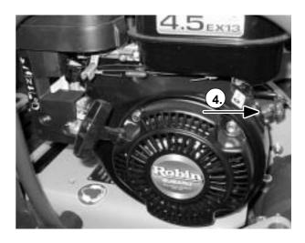
5. As the engine warms up (engine speed < 2000 min<sup>-1</sup>) gradually move the choke lever fully right to the OPEN position.
